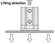
• Consider the center of gravity of the workpiece to avoid moments being applied to the magnet gripper as much as possible.
