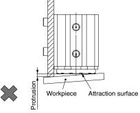
2. When multiple magnet grippers are used side by side, mount them so that the attraction surfaces are not uneven.
