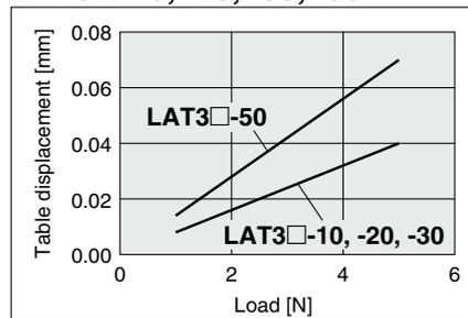
Table displacement due to roll moment load
