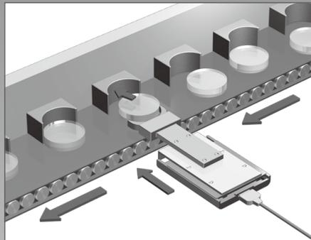
Cutting of resin mold component runners
