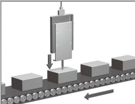
Measurement of glass substrate thickness (multiple points)
