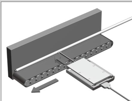
Measurement of tape thickness
