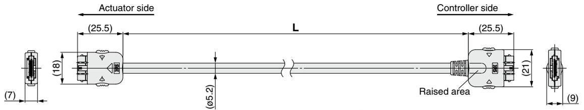
\* The actuator cable is direction dependent. Make sure to connect the Card Motor side of the cable to the Card Motor and vice versa. There is a small raised area on the connector for the controller.
