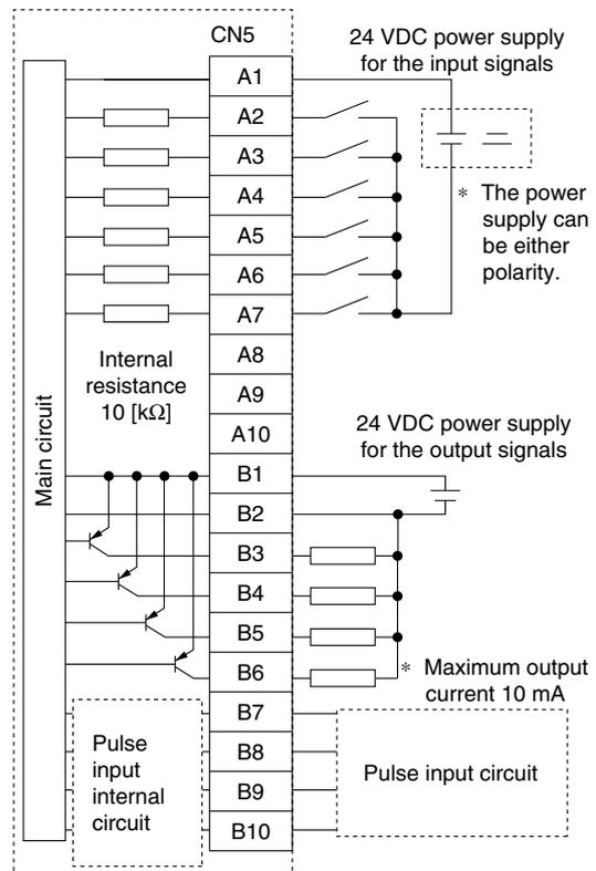
\* When using the controller by the step data input type, do not wire as there is an internal circuit to use terminals B7 to B10 as the pulse signal input terminals.
