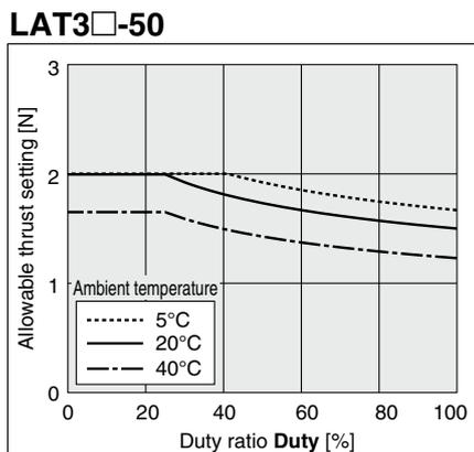
**Fig. 5 Pushing Force: F [N] Characteristics (Reference)**
