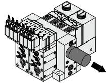
If there are a large number of ejectors that are linked on a manifold, which exhaust collectively, install a silencer at both ends. If the exhaust must be discharged outdoors through piping, make the diameter of the piping larger to control its back pressure to 5 kPa or less so that the back pressure will not affect the operation of the ejectors.
