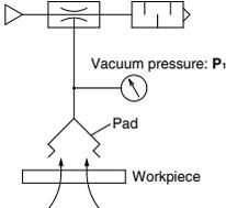
As described in the illustration to the left, adsorb the workpiece with the ejector, using the ejector, pad, and vacuum gauge. At this time, read the vacuum pressure  $P_1$ , obtain the suction flow rate from the flow rate characteristics graph for the ejector that is being used, and render this amount as the leakage of the workpiece.
