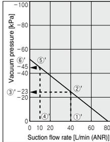
The vacuum pressure varies in accordance with the leakage volumes indicated in the above diagrams.
