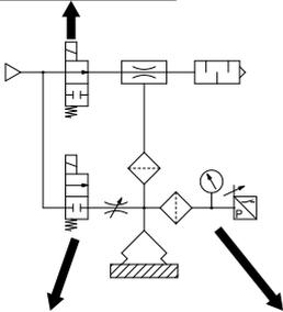
Be aware that the composite conductance consisting of the areas from the pad to the ejector of a vacuum switching valve does not decrease.
