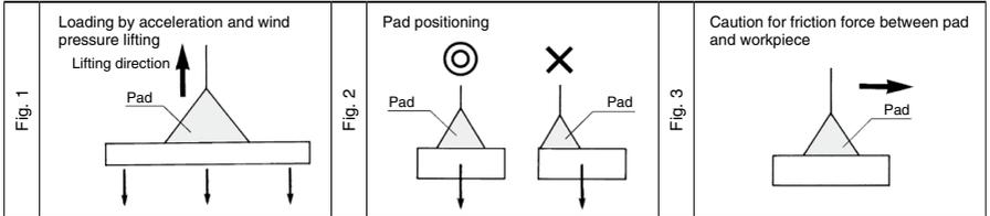
**Balance of Pad and Workpiece**
