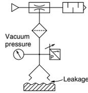
If a considerable amount of leakage occurs between the workpieces and the pads, resulting in incomplete adsorption, or to shorten the adsorption and transfer time, select an ejector nozzle with a larger diameter from the ZH, ZR, or ZL series.
