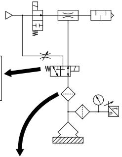
When using a 3-port valve, plug the exhaust port. When vacuum is generated, atmospheric pressure will flow in, resulting in decreased vacuum pressure.
